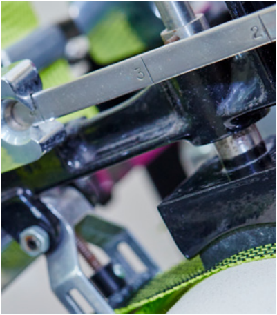
Above: Fabric being abraded in a Wyzenbeek machine
